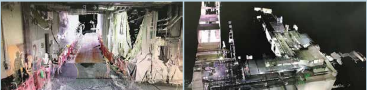
- 3D scanning for A&A works area to develop as-built point-cloud model for exact measurement
